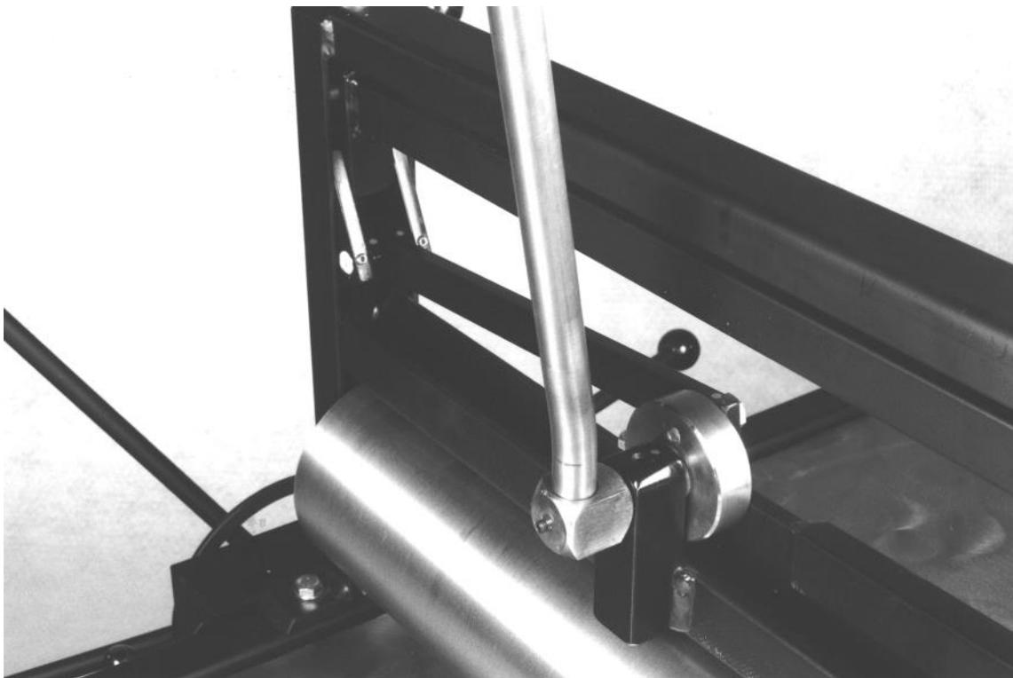
Moreover it is important to keep all polished parts/surfaces clean and dry to prevent them from rusting. The press must immediately be wiped off with a dry cloth if it gets wet.
