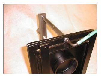
Place the two washers on the two M10 Allen screws and fasten the rods from the bottom with the M10 Allen key.
