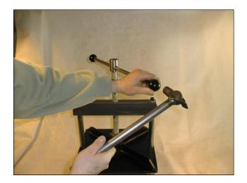
**6.** Assemble the handle by inserting the rod in the hole of he spindle. Fasten the loose ball onto the rod by hammering carefully.
