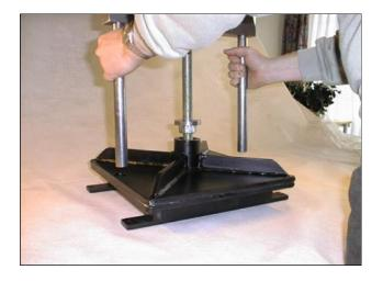
3. Place the rods of the upper part in the holes of the bedplates.
